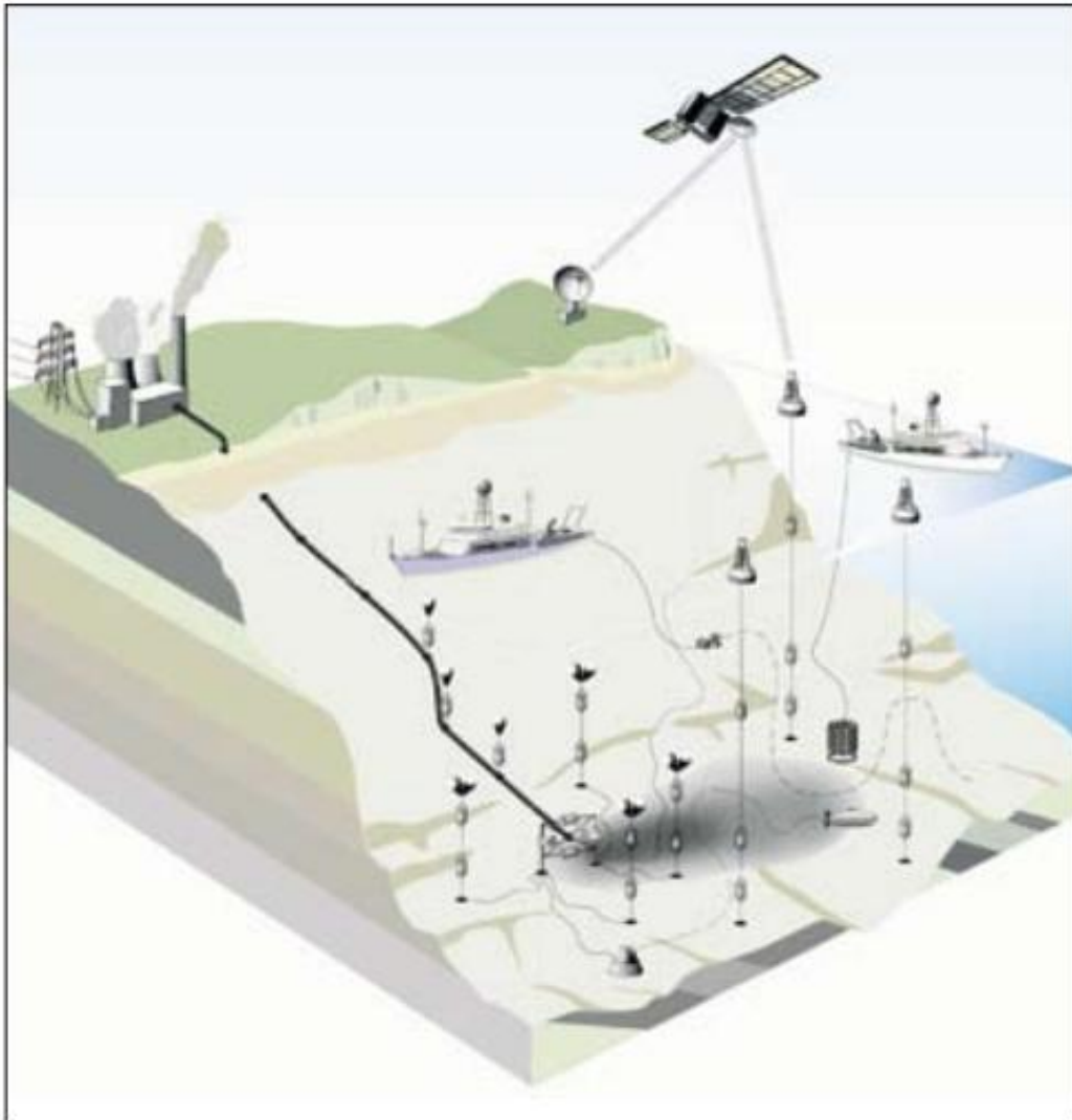
FIGURE 8-1: SCHEMATIC OF POSSIBLE APPROACHES FOR MONITORING THE INJECTION OF CO 2 INTO THE DEEP OCEAN VIA A PIPELINE. THE GREY REGION REPRESENTS A PLUME OF HIGH CO 2 /LOW pH WATER EXTENDING FROM THE END OF THE PIPELINE. SOURCE: IPCC (2005) FIGURE 6.22 ON PAGE 309.
